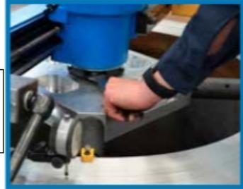
**3** Set the machine onto the flange.
