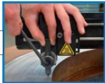
**4** Install the machining arm and slide to desired location.
