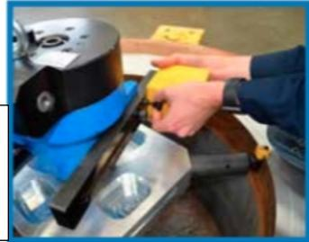
**2** Assemble the ID chuck and install appropriate leg spacers.
